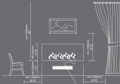
A power cable is required for connection to the mains. Specification - min. 3x0,75 mm<sup>2</sup>, with power supply 230 V, 50 Hz, to connect the device to the mains
