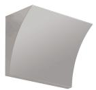
Wall lamp providing indirect light. Pressure die-cast Zamak alloy structure. Molded steel, galvanized white wall attachment containing the wall attachment system as well as the electrical devices. Pochette has a single dimmable light source in the traditional recessed series.
