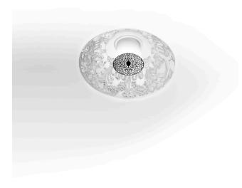
Recessed luminaire providing diffused lighting. Hemispherical, cast plaster diffuser, painted white inside. Plaster diffuser support in die-cast aluminum alloy. Flashed and blown opal glass diffuser. Frieze in photo-etched and mechanically drawn aisi 304 steel.
