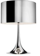
Table/desk lamp providing diffused light. Spun metal frame and diffuser, die-cast aluminum diffuser support arms and lampholder support, painted in the colors indicated below. White, injectionmolded polycarbonate diffuser supports. Sandblasted pressed glass upper diffuser screen.
