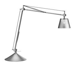
Task lamp providing direct and diffused light. Acid-etched pressed borosilicate glass internal diffuser. Injection-molded PC (polycarbonate) diffuser, vacuum-aluminized inside. Gray painted die-cast aluminum diffuser support. Gray painted assembly composed of extruded aluminum arms, steel tie rods, stainless steel springs, and 50% fiberglass reinforced, injection-molded polyamide joints. Gray painted die-cast Zamak BASE.
