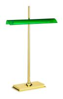
Table lamp providing direct light. Aluminium structure with external transparent methacrylate diffuser and opal PC led diffuser. Optical switch sensor on the base that provide 3-step dimming function. A USB socket on the back of the base enables you to recharge the most common smartphones and tablets (max 1.5A). Adaptor on plug connector with interchangeable plugs. The power chord is 2.5 metres long
